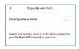
Go to **Settings – Capacity oriented Mode** in **My Mesh** app. Disable this mode when there are less than 30 clients connected to your WiFi at one time.
