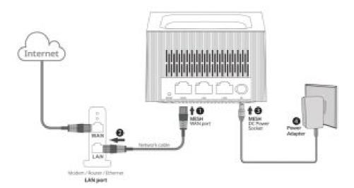
Turn on the power of the mesh and the indicator will become Green Solid. It will take about 45 seconds that the mesh to boot up completely till the indicator becomes Blinking Green.
