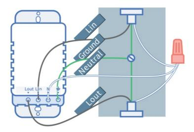
f) Push the smart switch back into the box and turn the power on at the circuit breaker. If the switch works manually and the LED is flashing amber and green, then you are good to go for setting up. If not, please turn off the power at the circuit breaker and check the wiring.
