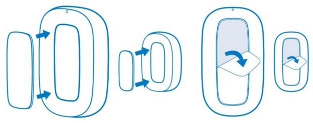
4. During installation, align the installation marking lines on the side of the main body and the magnet. Ensure that the surface of the installation location is clean and dry.
