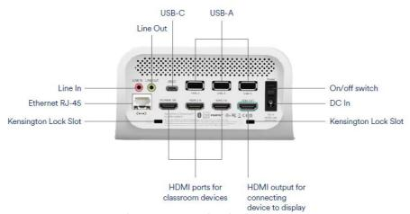
Total power supply up to 5V/2A for 3x USB-A and 1x USB-C .For interoperability with other devices, please refer to  $\frac{\text{merlyn.org}}{\text{support}}$ .
