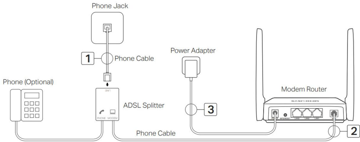
Wait about 1 to 2 minutes, then verify that the Power, ADSL and Wi-Fi LEDs are on before continuing.
