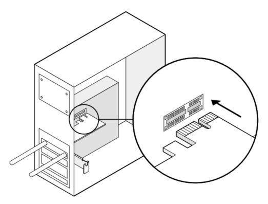
• d. Locate an available F\_USB connector and carefully plug the Bluetooth USB cable into it.
