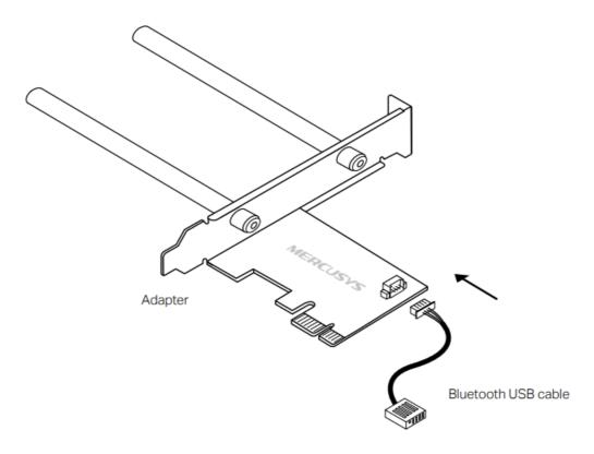
c. Locate an available PCI-E slot (X1, X4, X8, or X16) and carefully insert the adapter.
