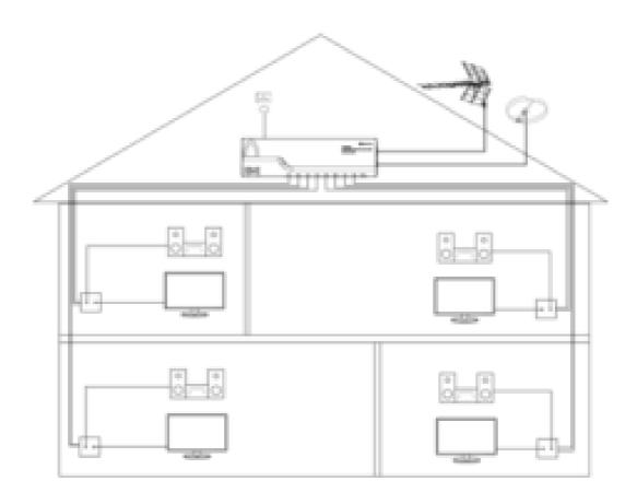
It is also suitable for upgrading or replacing existing UHF/VHF signal distribution units, simply reconnect the existing connector from the previous unit to the AMD amplifier. Ensure the UHF aerial is connected to the UHF input of the amplifier and FM/DAB aerials are connected to the VHF input of the amplifier. For loft distribution
