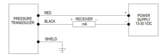
The maximum receiver load resistance (RLmax) for the DC power supply voltage (Vsup) is expressed by the formula:
