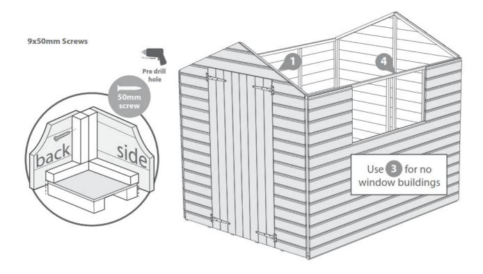
Place the ridge bar in between the front and back gables. Ensure the top corners of the ridge bar sit flush with the top points of the door gable. Fix the ridge bar to the gable using one L bracket for each end. Fix with 4x20mm screws each
