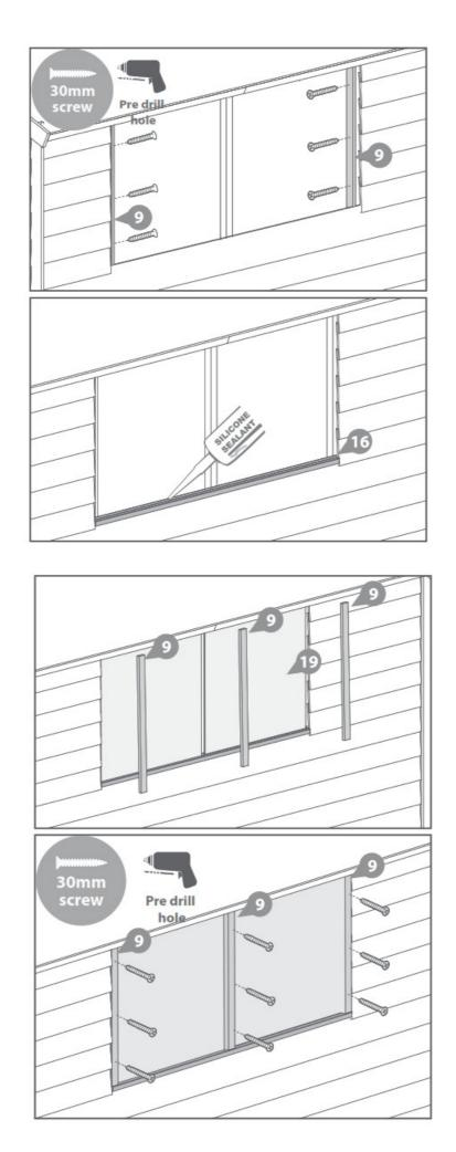
Fix the window strips to the two pieces of framing that sit alongside the outside edges of the window with 3x30mm screws for each strip.
