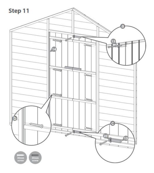
a First line up the door blocks at the top and bottom of the doors. Then fix with 2x30mm screws by screwing through the outside of the door into the block.
