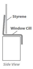
Place the plastic window cill onto the Window Panel and silicone in place as shown on both diagrams to the left.
