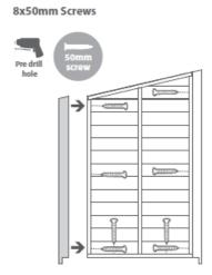
Place the remaining gable and front post onto the floor, align the gable with the inside of the rear post and secure in place using 8x50mm screws as shown in the illustration.
