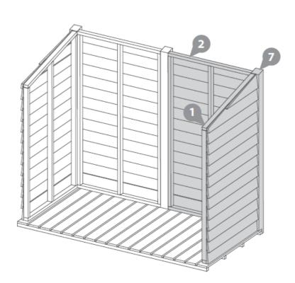
Following the same method outlined in steps 2 & 3 fix the second back panel and the right gable onto the assembly.
