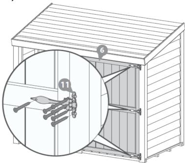
Place the door into the door gap and fix into place using 3x T-hinges securing each hinge with 7x30mm black screws.
