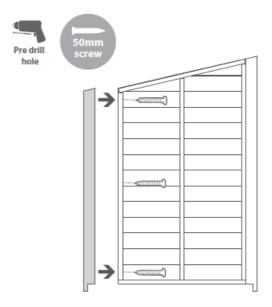
Attach the first 2 front posts to the building. Securing 1x post to each gable using 3x50mm screws.
