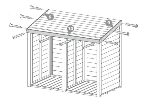
Attach the fascia's to the front and sides of the building, securing each fascia into place using 10x30mm screws. 10x30mm Screws
