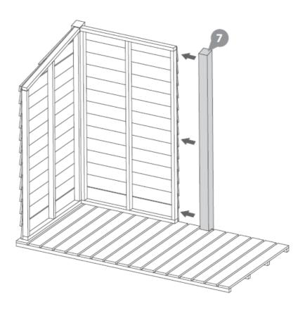
Attach the second rear post to the building, screwing though the panel into the post as shown in the illustration. \*Ensure the panel is flush to the inside edge of the post.
