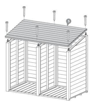
Place the roof on top of the building, aligning the roof so that it is flush with the rear. Secure the roof in place with 6x70mm screws as shown in the illustration.
