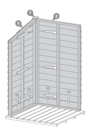
Place the first gable, back panel and rear post onto the floor. Secure each panel to the rear post using 3x50mm screws per panel.
