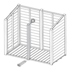
Place the remaining front post onto the floor, aligning with the rear post. Secure the post into place using 2x50mm screws, fixing through the front into the floor bearer.
