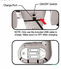
Your Robotosaur has a 3.7v 500 mAh rechargeable internal lithium battery. Although it comes with some charge, you need to charge it 60 minutes before use.
