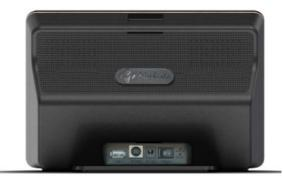
On the back you will find the USB port (for connecting USB flash drives for updates or PGN exports), the port for the chessboard, the power socket, the ON/off switch, the control led and the reset button.
