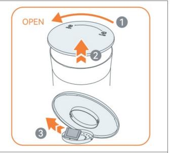
Twist to OPEN position to open the lid. Take out the de siccant bag.
