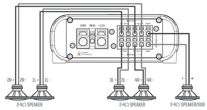
• WIRING 4-CHANNEL AMPLIFIERS – PRX500.4V2
