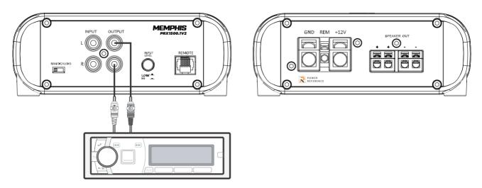
• WIRING 4-CHANNEL AMPLIFIERS - PRX500.4V2
