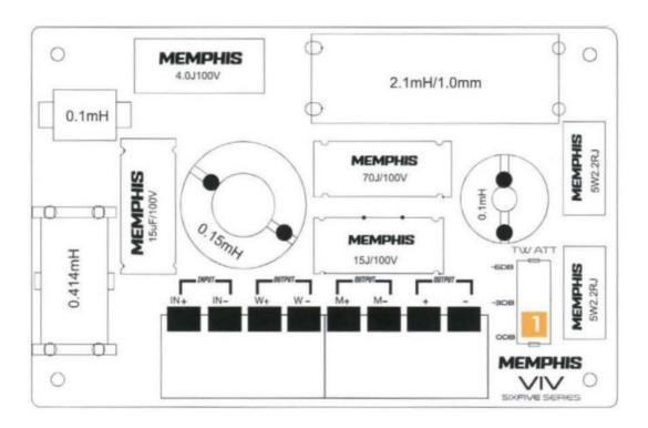
VIV603CV2 Crossovers uses switches to adjust a variety of features allowing the user to dial in the perfect sound for their audio system.
