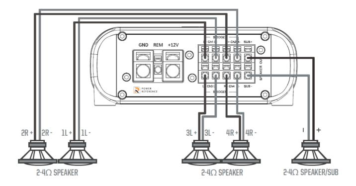
**WIRING 4-CHANNEL AMPLIFIERS – PRX500.4V2**
