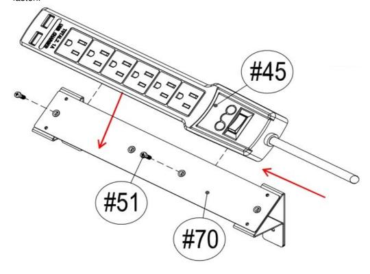
Note: The left and right directionsof PowerStrip can be interchangeable. Just tighten screws on the other twoholes. Pushitin opposite directiontofastenafter installing Power Strip.
