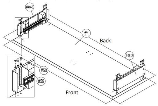
Note: Do not fully tighten any of thescrewsuntil all screws are partially screwedinfirst. Thiswill help you make any adjustments for alignment.
