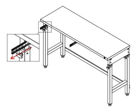
2. Attach and fit the Drawer to the innertrack of the sliders then slidedrawers in slowly.
