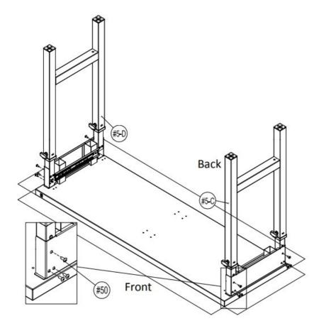
Note: Pay attention to the direction of the Left and Right Leg Piece, the screw knobs on the legs face out to the FRONT.
