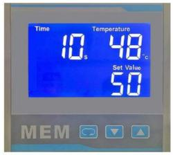
With the temperature controller, temperature (°C and °F) and pressing time can be adjusted. The Set values are showing the setting value, the Temperature digits are showing the actual value. The counter (reset after power off) function that counts the number of transfers that have already been made during the current session could be enabled, contact MEM for counter function enable instruction.
