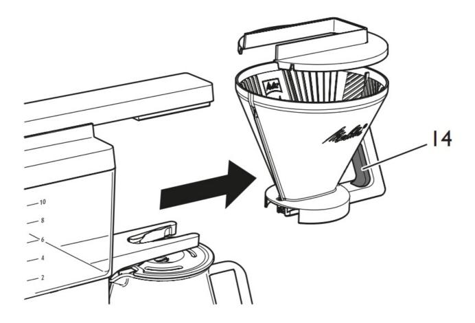
To remove the filter, press the lever (14) and pull the filter by the filter handle out of the appliance.
