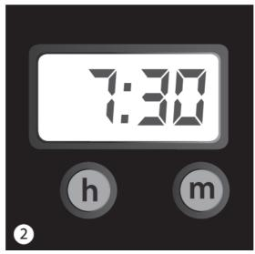
. This goes faster if you hold down the button. The appliance is only ready to use once the time has been set. You can turn the display light on or off by simultaneously pressing the h and m buttons 3
