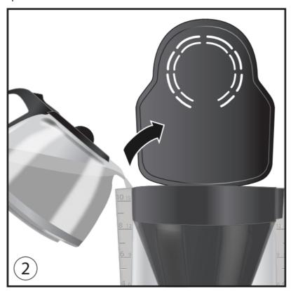
• Fill the water tank with the desired amount of water using the glass pot. With the help of the water level display on the tank 3 you can choose the correct number of cups.
