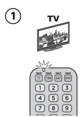
2. Press and hold the button until the top LED lights up. Release the button.
