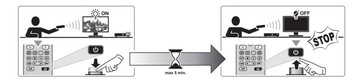
Point the remote control at the device, hold down the but, ton and release it as soon as the device switches off (max 5 minutes)
