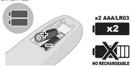
Press and hold button 5 and check that the LED on the remote control remains continuously lit until the button is released. If the LED flashes or stays off the batteries used are not sufficiently charged: replace them.
