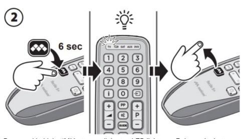
Press and hold the "M" button until the top LED lights up. Release the button.
