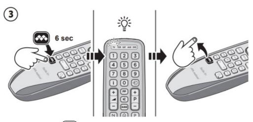
Press and hold the button until the top LED lights up. Release the button.
