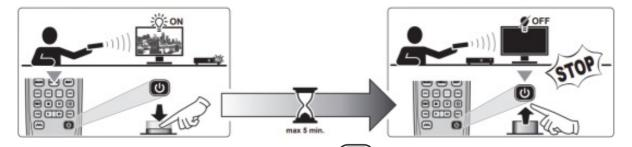
Point the remote control at the device, hold down the button and release it as soon as the device switches off (max 5 minutes).
