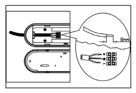
4. If using a cable gland, turn the sealing nut clockwise to ensure proper ingress protection of cable.
