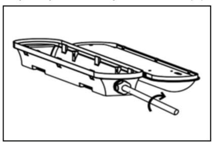
5. Close the fitting by re-installing the clips, ensuring that the diffuser properly mates with the fitting gasket to maintain ingress protection.
