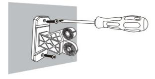
• Step 3: Turn on the switch of the lamp, set the mode and angle of the lamp, and then tighten the screw to fix the lamp on the mounting base.
