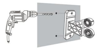
• Step 2: Drive in bolts and screws to fix the mounting base on the wall.
