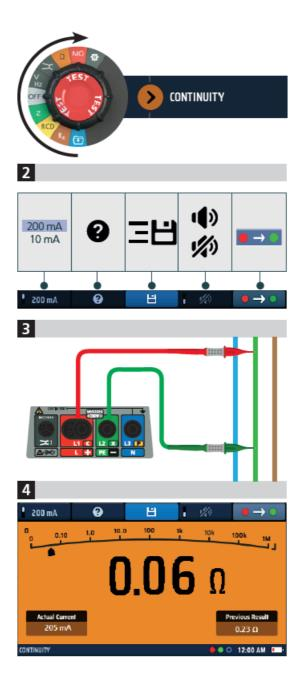
Test Lead Null (Ω)
