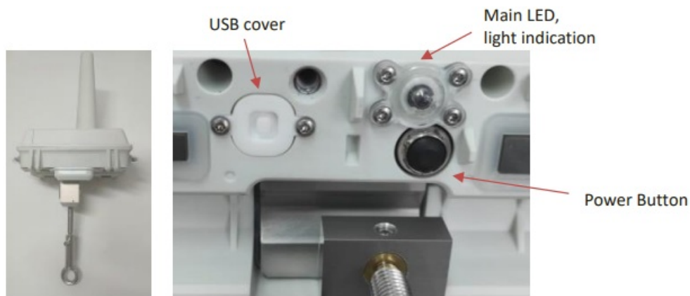
Figure 5: USB cover, Power Button and Main LED
