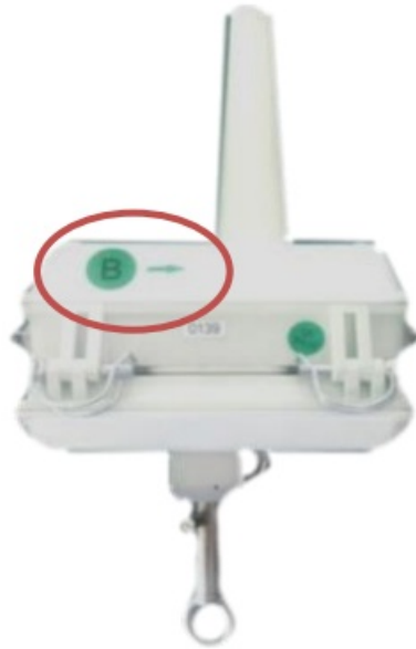
Figure 19: Phase and power flow arrow labels
