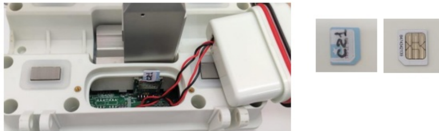
Figure 3: Inserting micro-SIM card into SIM socket
