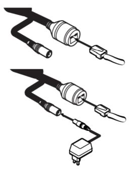
2. **NETWORK CONNECTIONS** – Not using PoE Switch or PoE Injector, connect the camera to the switch using an Ethernet cable for data transmission and use a power adapter to power the camera.
