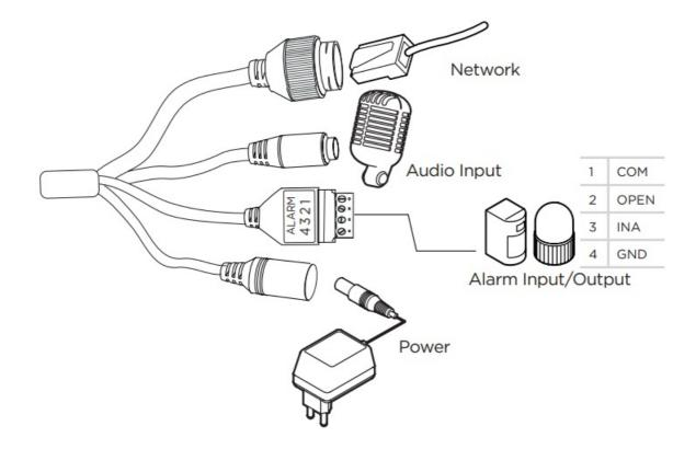
Use the diagram below to properly connect power, network, alarm input and outputs and audio to the camera.
