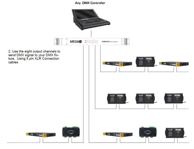
2. Use the eight output channels to send DMX signal to your DMX fix-ture. Using 5 pin XLR Connection cables
