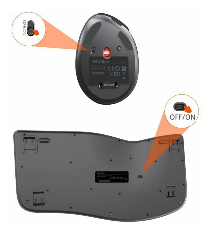
Toggle the switch at the bottom of the device to "ON"
