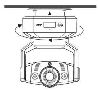
Push the camera against the mounting plate and rotate it clockwise. Caution: Always hold the camera by the base and avoid touching the lens
