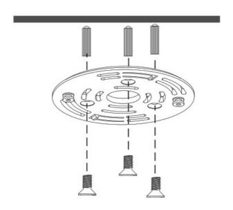
Use the included hardware to attach the mounting plate to the ceiling as shown. Point the arrow on the mounting plate in the direction you want the camera to face.
