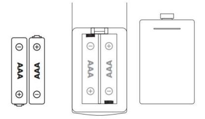
Install 2x AAA batteries in the battery compartment located on the back of the remote control Note: Batteries not included
