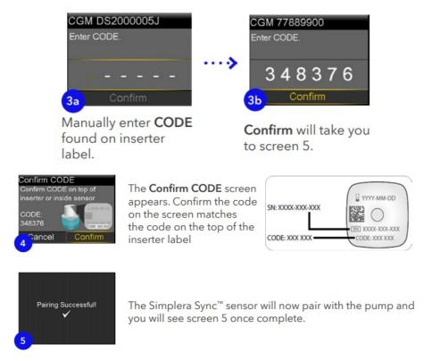
**NOTE**: Step 1 is only required when using a Guardian<sup>™</sup> sensor/ transmitter. You do not need to unpair anything when starting your next Simplera Sync<sup>™</sup> sensor; just pair your new one and the old one is disconnected automatically.
