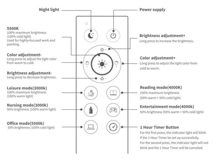
**Night light mode:** The power rate of night light mode is only 8 %0 of the usual brightness mode. You can turn on night light mode simultaneously while the light is off, and turn off the night light via any keys.
