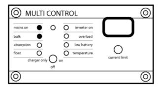
• Bulk/Absorption Charge: The unit has AC input voltage and is bulk charging but not yet reached absorption voltage yet.
