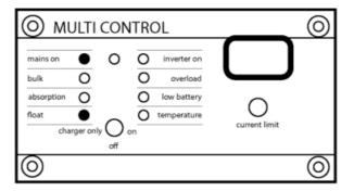
• **Equalize Mode:** The unit has AC input voltage and is equalizing battery bank while passing the power through to the equipment load:
