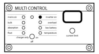
• Excess Overload: The equipment load is exceeding the unit's regular output, reduce the equipment load:
