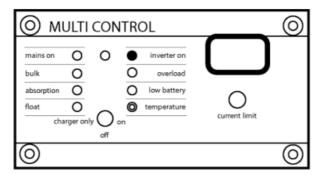
• **Temperature overload:** The unit has reached an internal temperature level that is too high, and the unit shut off:
