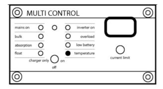
• Battery voltage too high: The unit's battery voltage is too high; be sure the correct batteries are being used and they are installed correctly.
