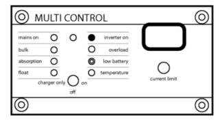
• Batteries are dead: This indicates that the battery voltage had gone too low, and the inverter has switched off.
