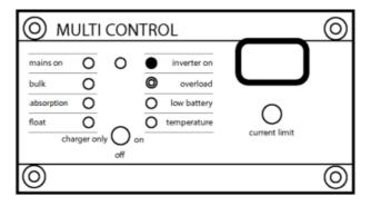
• Overload: This indicates that the unit is overloaded due to either a short circuit on the output or the equipment load is too large for the system to support:
