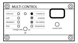
• Erratic battery voltage: The unit shut down due to excess ripple voltages out of the battery.
