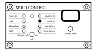
• Batteries are low: This indicates that the system batteries are low. If the unit is supporting a load, it will not be long before the batteries go dead:
