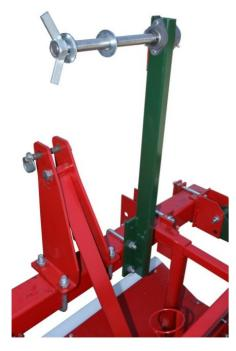
2. Bolt tape guide to 2 x 2 bar on main pan using 2-1/2 x 3-1/2" bolts. Slide tape guide bracket on bar to the desired offset and tighten bolts.
