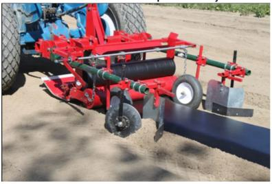
Mount green round side arms onto above clamps. Use  $2-3/4 \times 5$  bolts and 3/4" lock nuts. Tighten snuggly just so green sidearm can move freely up and down.
