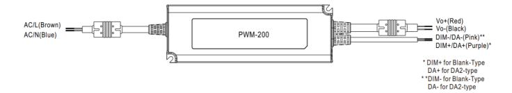
Dimming principle for PWM style output Dimming is achieved by varying the duty cycle of the output current.
