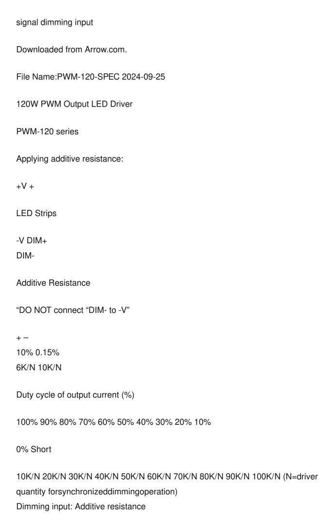
Note: 1. Min. duty cycle of output current is about 0.15%, and the dimming input is about 6K or 0.6VDC, or 10V PWM signal with 6% duty cycle. 2. The duty cycle of output current could drop down to 0% when dimming input is less than 6K or less than 0.6VDC, or 10V PWM signal with duty cycle less than 6%.
