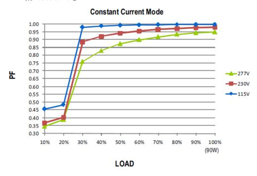
De-rating is needed under low input voltage,
