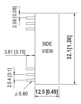
NOTE: Pin tolerance ±0.5mm
