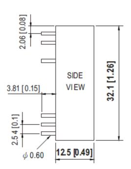
NOTE: Pin tolerance ±0.5mm
