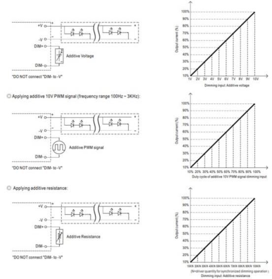
**Note:** In the case of turning the lighting fixture down to 0% brightness, please refer to the configuration as follow, or please contact MEAN WELL for other options.
