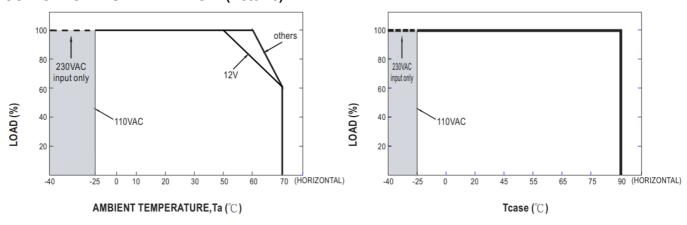
• If ELG-200 operates in Constant Current mode with the rated current, the maximum workable Ta is 50 °C for °C
