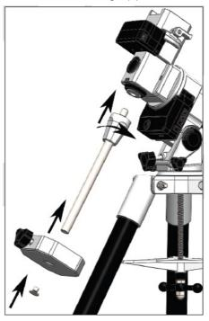
• Step 7: Install the Optical Tube and secure with 2 locking knobs.
