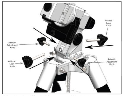
• Step 5: Adjust to local latitude using Altitude Adjustment and Lock Knobs
