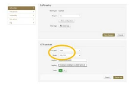
Now the device is registered in our OTA devices list. After the join we can see the details of the device by clicking on the search icon.
