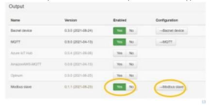
Second step is to set the port on 502 for modbus slave communication.
