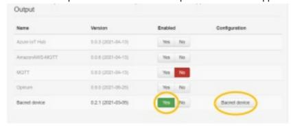
When we click on enable "YES" a BACnet device configuration button appears. Clicking on this button takes you to the BACnet settings page.
