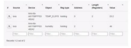
The registers are "03 registers" (read holding registers)16 bits.
