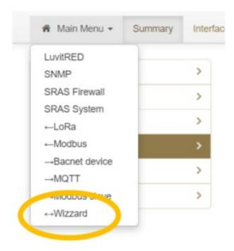
The LoRa-2-BMS Wizzard can be used to connect sensors and devices of different interfaces and/or protocols. The list below gives an overview of the currently supported Input interfaces and/or protocols:
