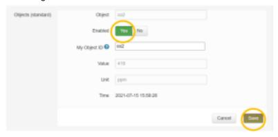
The last step is to enable the Data upload and press save.
