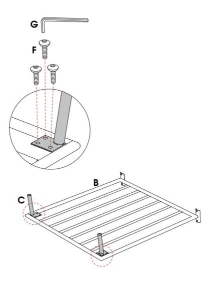
**Step 2**Combine the Back Frame #A with the Seat Frame #B using 4 screws #F as shown and tighten the screws by Allen Wrench #G.
