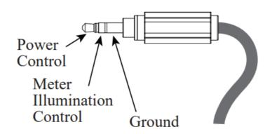
Meter illumination can also be controlled via the Power Control Input's source.
