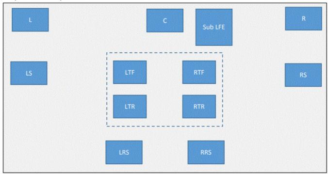
If Auro-3D material is played on this setup, the system will play the HL/HR channels through the LTF/RTF speakers and the HLS/HRS channels through the LTR/RTR speakers. The LRS and RRS speakers will not be used.
