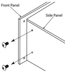
2. Secure the rack mounting bracket to the MIP200 side panel using 2 of the 8-32 thread (larger) flathead screws. Do not re-use the previously removed screws. Use 2 of the supplied 6-32 thread (smaller) flathead screws to secure the bracket to the front panel.
