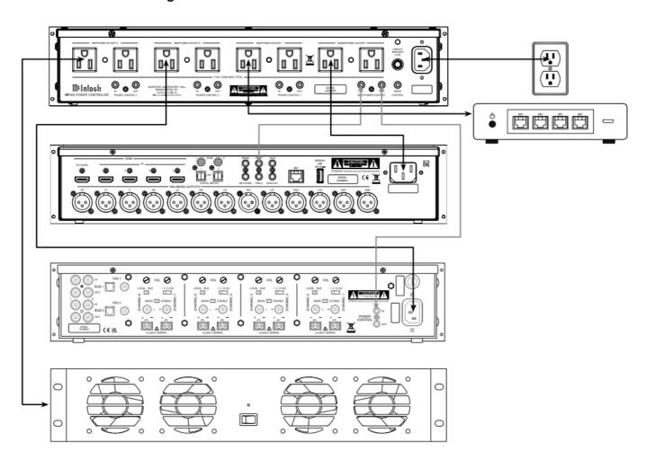
• In this connection example, a home theater processor, power amplifier, network router, and equipment rack fan are shown connected to the MIP200.
