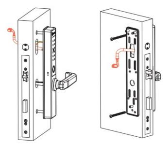
· Remove the interior lock assembly, then tighten the two screws.
