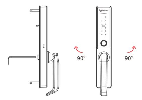
1. Rotate the handle 90 degrees to the left or right and re-tighten the screw.
